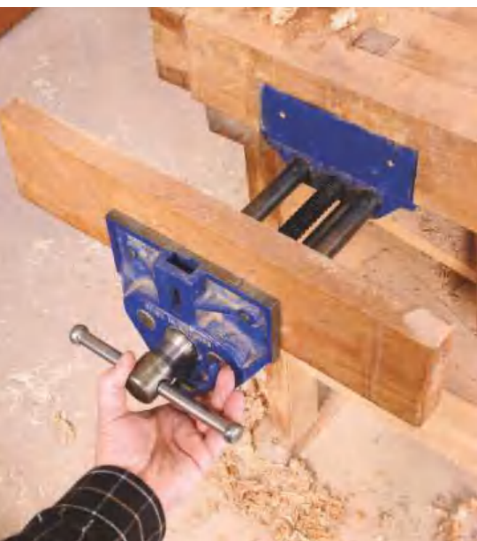
▲ Pic.7 The bench vice is a necessary tool to grip wood while sawing and planing
